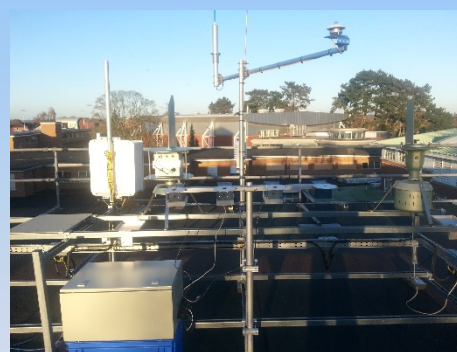
Setup showing rotating, fixed OPCs and ordinary Burkard trap
