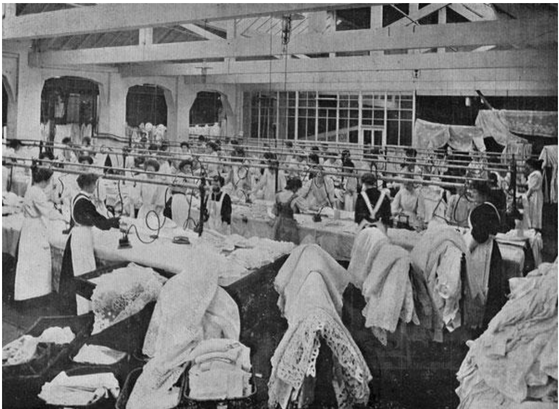
Area showing ironing of small items using gas-powered irons.
