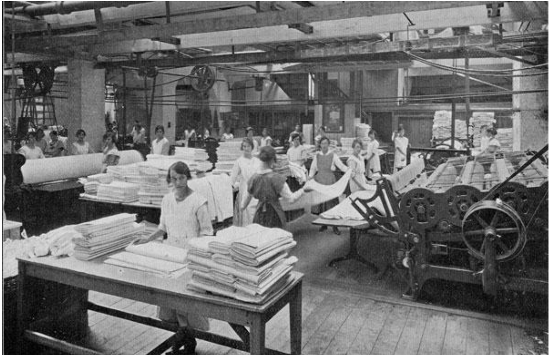
Area showing large for drying and pressing sheets and table linen, powered by steam, with unguarded belts and pulleys.
